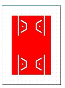
Click on the downward facing arrow to the right of the selection boxes to launch the different options. Set the **Material** to Acrylic (Cast). As we are using a 3mm tool, set the **Edging Tool** and **Area Tool** to 3.
