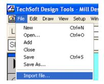
A popup menu will appear from which you must choose the file location. The type of file that we require is a .DXF file. Select the drop down arrow to the right of the box for File of type: This will produce a drop down menu from which you can select DXF Files. Find the file Flat pattern\_Folded Chassis.DXF and select Open.
